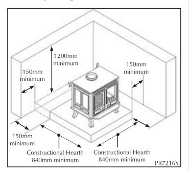
If you are fitting the appliance into an existing hearth setting check that it complies with the current construction regulations and is at least the minimum sizes shown.
